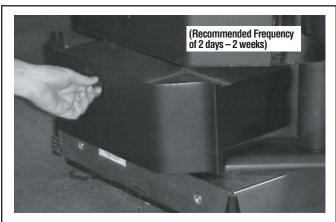
Figure 46 - Ash Pan, Profile 20 FS-2 and Profile 30 FS-2
